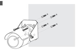
Installing using Wall Mount
